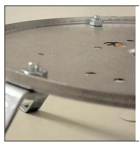
STEP 8: Attach Burner to Burner Brackets. **Pilot Orifice MUST face** toward the Control Assembly! Secure burner to brackets with 1/4-20 bolts and nuts.
