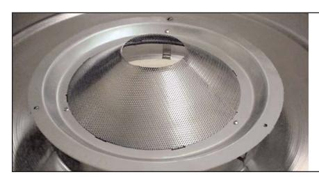
**STEP 6**: Attach reflector pan and insert 10-24 x ½ screw into set of 3 holes closest to glow housing perforation. Attach 10-24 nut and tighten.
